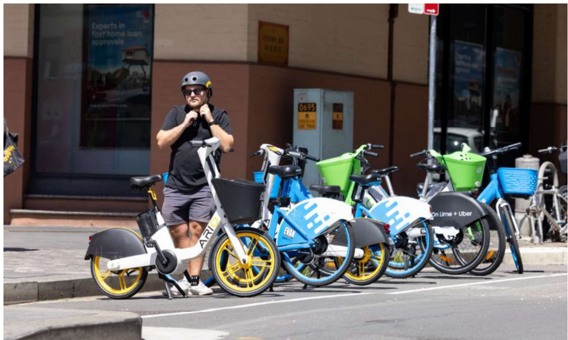
Figure 15 Dedicated on-street shared bike parking located in Ultimo Street, Haymarket. Note the white edge line to delineate the parking area. As the adjacent kerb build-out encourages perpendicular orientation of parked bikes, no racks are provided
